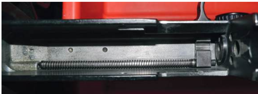
Cocking handle recoil spring and guide rod assembly in place.
