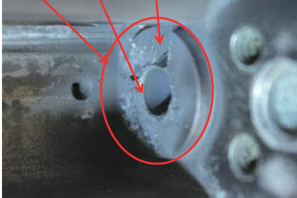
Ruger 10/22 chamber face showing fouling.
