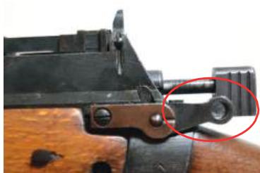
Safety Catch – applied. Rifle is cocked
