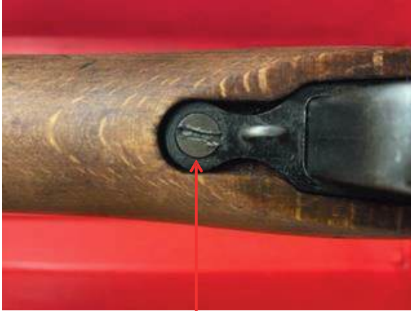
Damaged bedding screw on a No.4 Enfield
