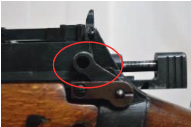
Safety Catch – not applied. Rifle is cocked
