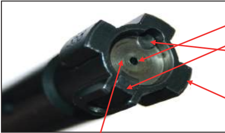
This machined out area of the bolt nose is called the bolt face recess
