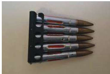
Drill rounds correctly placed into the charger.
